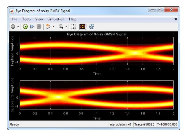
The eye diagram plot now renders accurately because the histogram interpolation method works for all SNR values. This method is not as fast as the other techniques and results in increased execution time.
