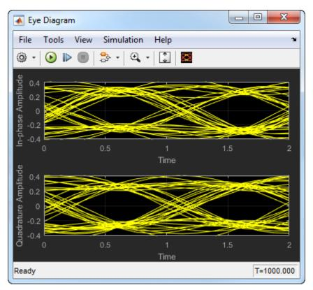
Open the configuration parameters dialog box. Change the **Symbols per trace** parameter to 4. Run the simulation and observe that four symbols are displayed.
